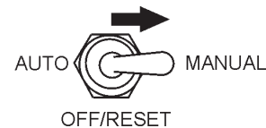
Figure 41. MPEC Control Switch (Manual Position)
